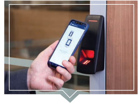
Identification by smartphone with NFC-module cards
